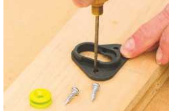
Mating brackets are fitted with 4.5mm pan-head screws
